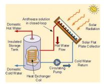
Active solar heating systems use heat pumps to transfer the collected heat from solar collectors into the building for storage or use.
