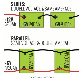
Number of 250Ah Lead-Acid batteries (with 50% discharge) = 750 Ah / .50 = 1500 Ah / 250 Ah = 6
